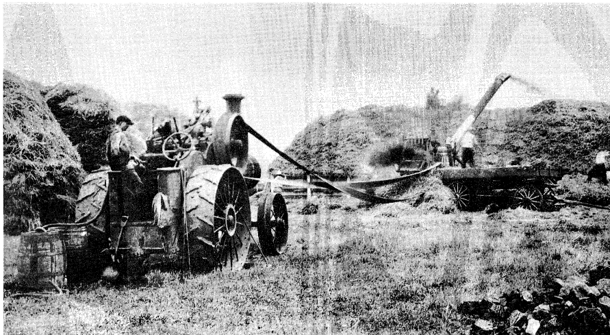
Figure 8: Self-propelled steam engines were extensively used during the latter part of the 19th century for operating grain-threshing machines and other stationary farm machines such as corn husker-shredders and shellers.
