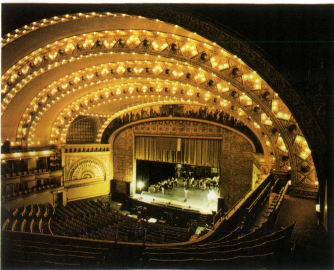
Auditorium of the Auditorium Building, Chicago, by Dankmar Adler and Louis Sullivan, 1889, renovated 1967–68: horseshoe-planned theatre with boxes and sloping galleries engineered for acoustical perfection and advantageous sight lines.
